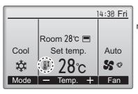
will appear on the Main display in the Full mode when the temperature range is restricted.
